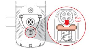
2. Push down the handle direction changing lever which is located After push down, the handle direction changing lever and rotating the handle in the desired direction from the handle turned back to the center, it will be fixed with a "click" sound.
