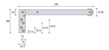
Application: used on double doors to control the sequence of door closing
