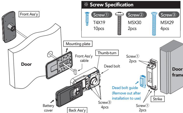
4. Front ass'y cable insert to back ass'y connector. Fix at the mounting plate by using fasten **screw ③**.
