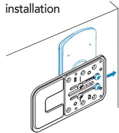
1. Tighten the screws(M5\*30) to the front Ass'y by 10mm first (based on 40mm of door thickness)
